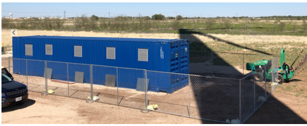
Figure 2: First auto transformer based test devices in USA at test side of GE. With this test device probably the first medium voltage OVRT test on a turbine level in America was successful carried out in May 2019.
